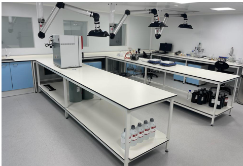
Production lab with Trespa fixed lab benching
