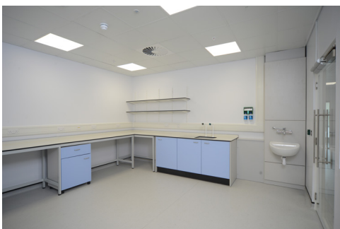
Super small lab with perimeter benching & IPS unit
